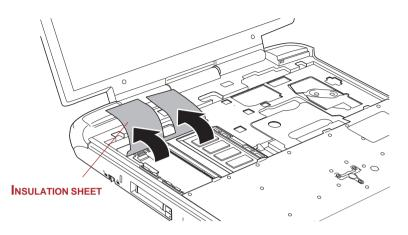
Figure 8-11 Raising the insulation sheet
